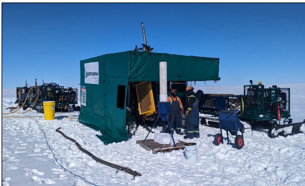
Reverse Circulation (RC) drilling with the track-mounted rig underway at Cyclone North, Storm Project, Nunavut.
